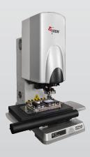
**VIEW Benchmark**<sup>™</sup> **250** is a compact, rugged, benchtop metrology system with all the features and capabilities of the larger VIEW models.
